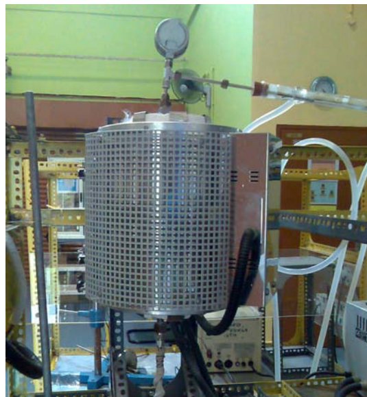
Fig. 1: The reactor is heated inside this tubular furnace which is part of the experimental set-up of the reaction
